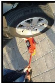
Raise the vehicle enough to remove the lower the lifting jack.
